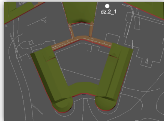
Figure 10 - Comparison between model from historical map and current base map (shifts and scale error)
